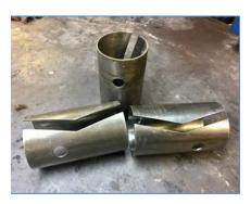
LANG'S TECH TIP! To determine the right from the left sleeve - hold the sleeve so you are looking at the V-slot and the slot points down. If the hole is on the right it is the right sleeve - if the hole is on the left it is the left sleeve.
