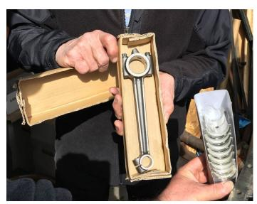
New Model T rods and shell bearing to go with the Scat crank Chris is installing in his new T engine project.
