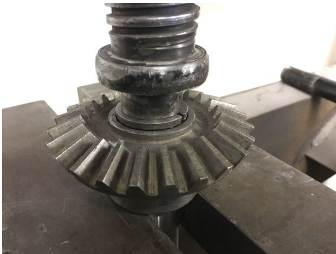
Seating the gear on the new axle
