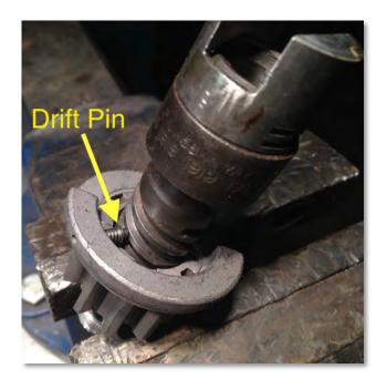
The Bendix assembly is connected to the starter shaft through a spring, which uncoils absorbing the initial torsional impact of the spinning starter and then rewinds applying its energy to help crank the engine.
