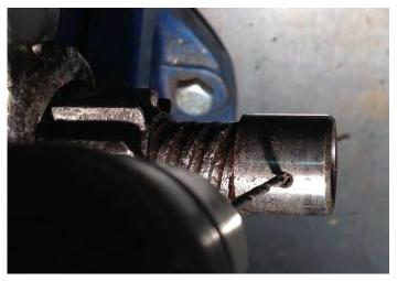
become separated from the pinion gear. These were often welded or brazed back in place. I repaired a couple of these gears only to find that the drift pin hole was out of alignment and the pin would not ride on top of the helical thread. New gears are not that expensive.
