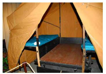
The campers built in the teens and early twenties shared a common design: a wooden trailer box with slide out or flip out beds; all covered with a tent that draped over the assembly and hung to the ground. Later more complex designs appeared with hard tops and spring loaded mechanisms that unfolded quickly with a minimum of human intervention. A few companies even supplied motorhome conversions which were designed for the Model T Chassis.
