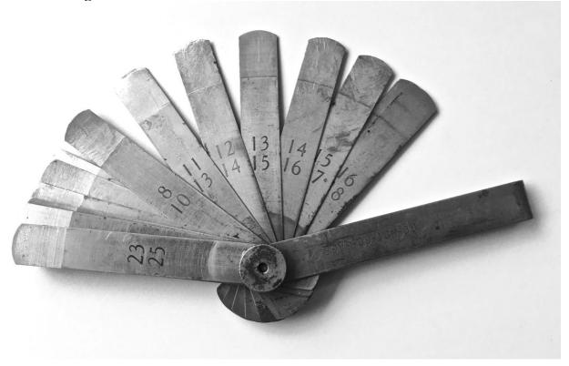
A common way to measure valve lash is with a feeler gauge. While shopping with Peter Anderson at a used tool store I came across a couple of stepped gauges referred to a "go-no-go" gauges. The stepped gauge lets you know when you are approaching the target valve clearance, speeding up the job of adjusting the valves.
