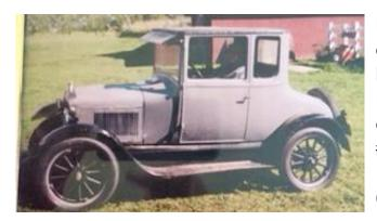
For Sale: 1926 Grey & Black Model T Coupe. Another one of Howard Majury's many Model Ts. Untouched, but new wiring, Has a Ruckstell transmission. Howard's note suggests "should have engine overhaul". Block Serial # C404980 (1913), Frame Serial # C697091 (late 1925). Filmed in the movie 'After the Harvest' in Bragg Creek. \$6000 OBO Phone or text 403-652-6233 or e mail <a href="mailto:chowridge@hotmail.ca">chowridge@hotmail.ca</a>
