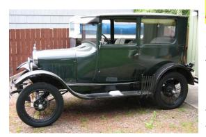
sold 1927 Model T Tudor \$9,500 It is a driver, not a show car. It is our 'go to' car for most tours as it has windows and is the most comfortable on cold mornings. This is a car you can enjoy immediately, and drive as is. Has a six-volt electric starter. The engine is equipped with a distributor which was a common period accessory. The two-speed planetary transmission is paired to a Ruckstell two-speed rear axle. Is equipped with Rocky Mountain
