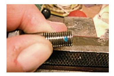
Spin the un-drilled hex-nut all the way down the shank of the bolt and screw on the drilled nut. While looking through the hole in the side of the nut, find the magic marker
