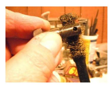
Don't remove the hex-nut just yet. Clean the threads up with a wire brush and then spin the hex-nut up
