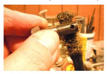
and down the bolt to chase the threads. Take the hex-nut off and finish cleaning up the threads with the wire brush.
