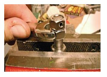
Clamp the stuck-together bolt & nuts unit into your vice, poke your drill-bit through the hole in the side of the nut and drill a little more than halfway through the bolt.
