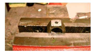
Measure the spot on the bolt where you want to put the cotter-pin hole and put a dot there with a magic marker.
