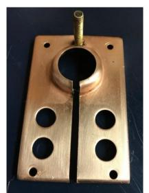
I posted a question on what I thought to be 'Copper topped' coils on the MTFCA Forum – "What is history on Copper Topped coils vs Brass topped coils? Should the copper be 'just copper' in appearance? polished? clear coated? They appear to be less in numbers from what I've seen when collecting 'metal topped' coils. Thoughts??" – Turns out they are all Brass- just 'yellow or red' brass.
