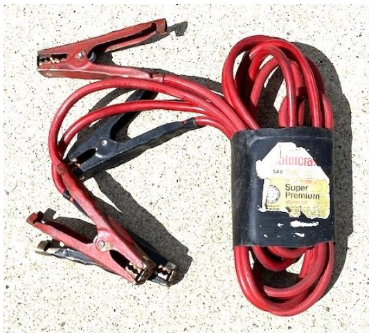
Here is a smart way to store those unruly battery cables. A 1-liter oil container with both ends removed slid over a looped set of cables.
