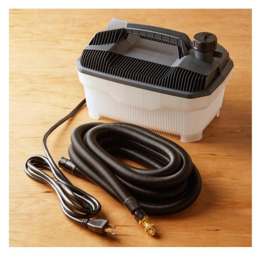
Les Schubert bought and showed an Earlex Steam Generator for a Wood bending unit that he thought the club should add to our tool collection. Steam bending is the process of soaking a piece of wood in hot water at a boiling point for a certain period of time in a steam box, softening the fibres to make it pliable and "stretchier," Once the timber cools down and the fibres dry once more, it will retain its new shape.
