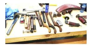
Day 3 – Metal Finish Repair on Automobile Bodies: using minimal tools showed how to return metal to original contour without use of filler. Focused on shaping and welding. Talked about the tools and accessories, assessment of damage and corrosion, minor impact repair, metal shaping and welding, fill repairs including dent repair, body soldering,
