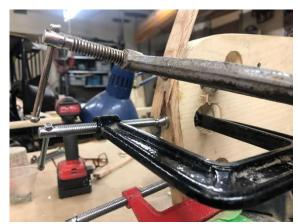
Wood fibres will not stretch but they will compress. For the more extreme bends, I screwed wood stops to a metal strap, allowing just enough room between the stops to tightly capture the oak. The strap was attached to the fixture. I then steamed the wood for about 30 minutes and quickly fixed it in my jig. The setup worked like a dream.
