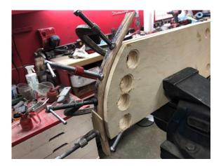
My first attempts were made after soaking the wood overnight in water mixed with fabric softener. I then steamed the wood for an hour and attempted the bends. The mild bends worked fine but the more extreme bends failed.
