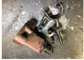
It is best not to do this on the kitchen stove, or your house will smell like greasy car parts and you will be sleeping in the garage. I simmered these parts for 30 minutes in tap water seeded with two Cascade dishwasher pods. The brew did a good job of removing the sludge and most of the paint.
