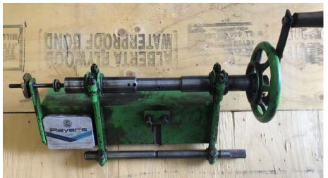
A Connecting Rod Boring Jig
